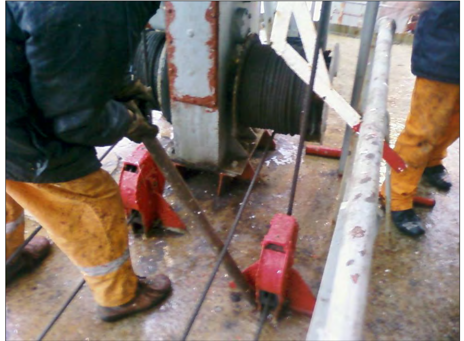
Crew manually guiding wire rope onto drum
