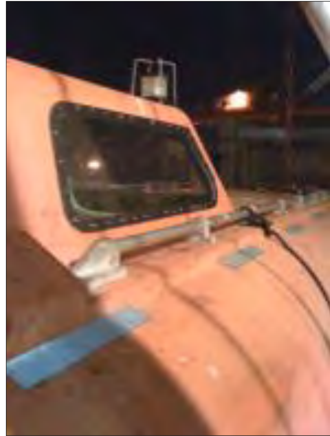
Life Boat windows obscured or opaque – before and after
