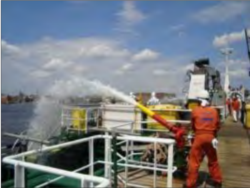
Insufficient fire main pressure – emergency fire pump wired backwards
